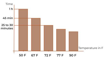
Drying times are affected by temperature and relative humidity. The chart represents guidline values but each project is to be treated individually.
